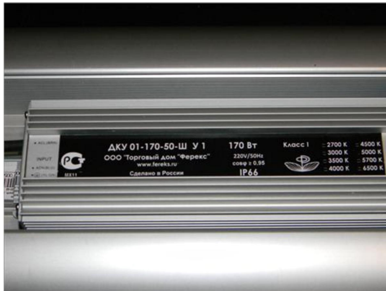
Figure 7: Picture of LED driver
