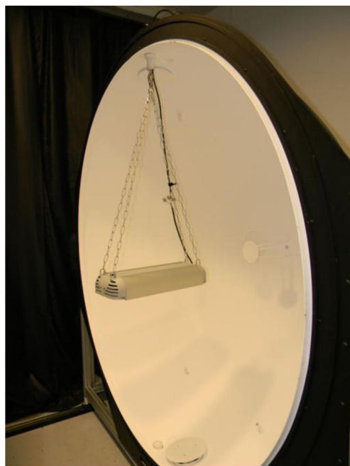
Figure 3: Sample in 2m Integrating Sphere
